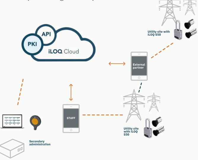
The iLOQ S50 is part of the digital ecosystem and is fully equipped to securely integrate with mobile devices. The phones collect and send real-time audit trails automatically to the cloud.
