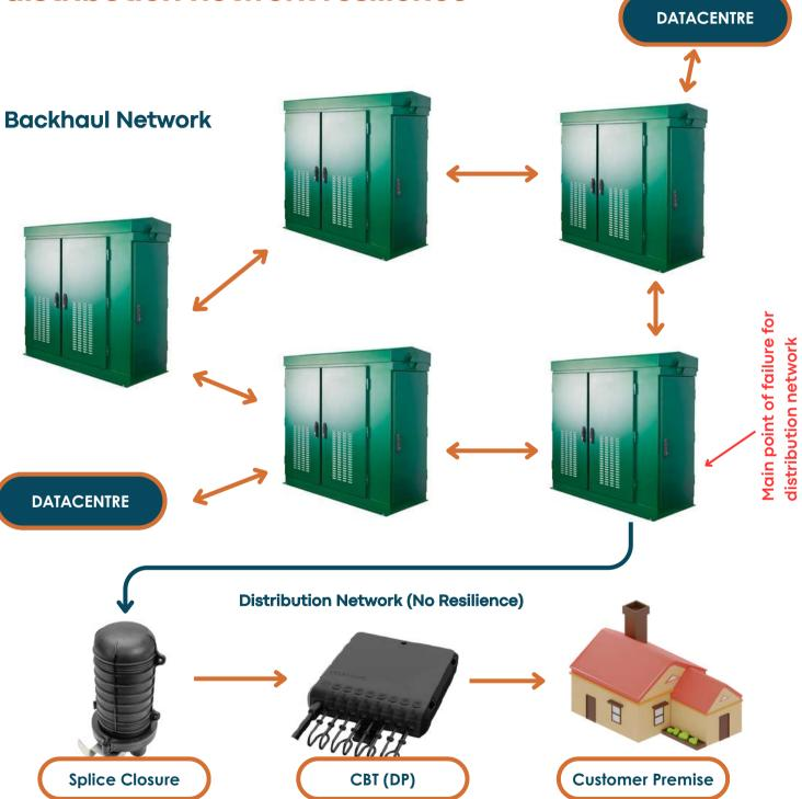
Securing and monitoring street cabinets is crucial, as issues within them could impact thousands of customers as the customer base grows. Despite improved backhaul network resilience, each cabinet remains a single point of failure for all customers it serves.
